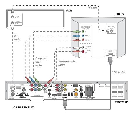
In Setup 1, connect your set-top to your TV via **either** an HDMI connector, **or** via component video connectors.
