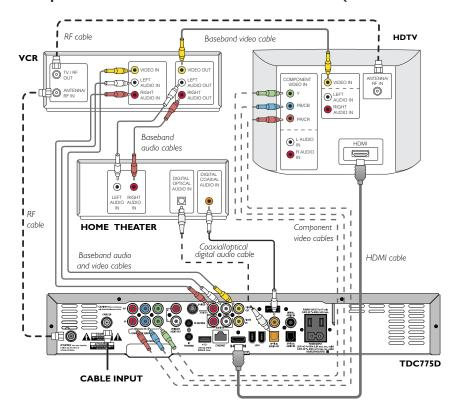
In Setup 2, connect your set-top to your TV via **either** an HDMI connector, **or** via component video connectors.
